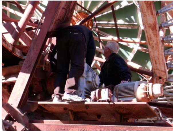
Expert inspection of a Declination drive
