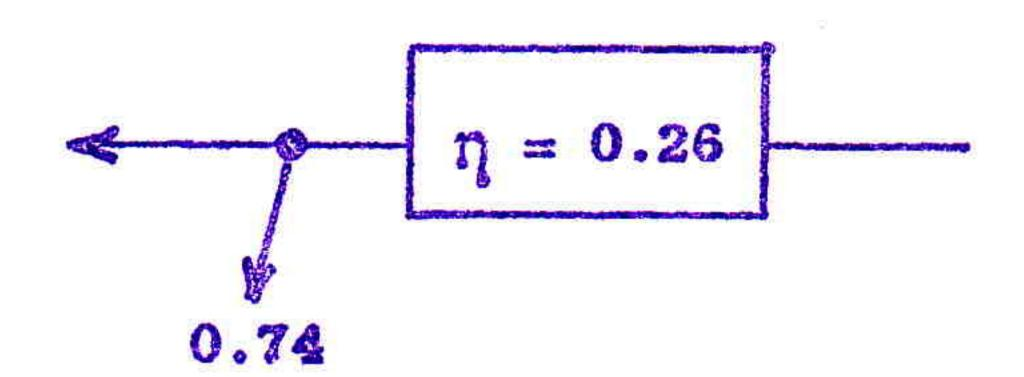
The oil churning loss is assumed to be the same because the gearing speeds are the same. The efficiency is calculated from  $(2 - 1/\eta)(2 - 1/\eta_2)$  where  $\eta_1 = 0.7$  and  $\eta_2 = 0.64$  are the forward efficiencies of the two stages (Glint 330, App. 5).
