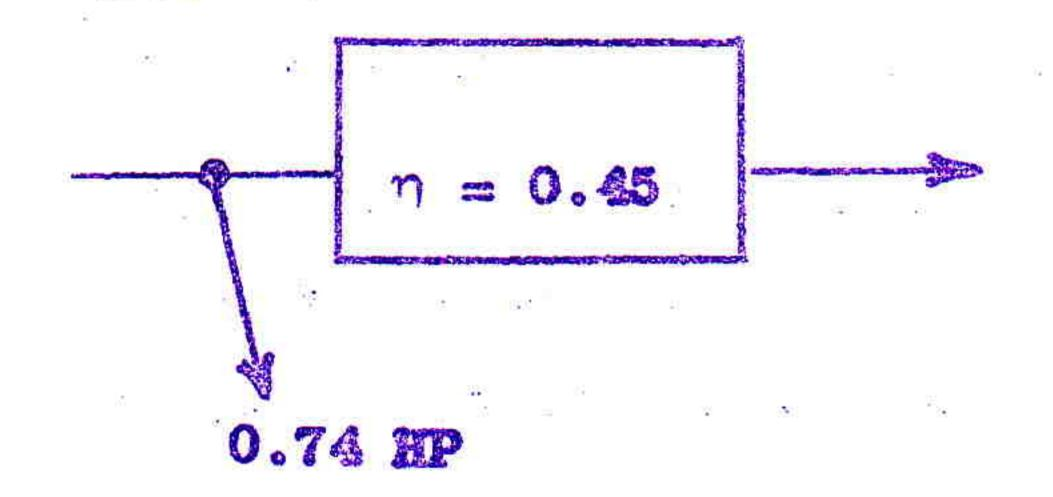
An oil churning loss of 0.74 MP is adopted, regardless of load, in accordance with measurements reported in Glint 330. Hore recent indications (of about 6 August 1969) are that this loss fell to 0.5 MP when the oil level was lowered to recommended level. Some further drop may possibly be expected from the use of a lighter grade of oil.
