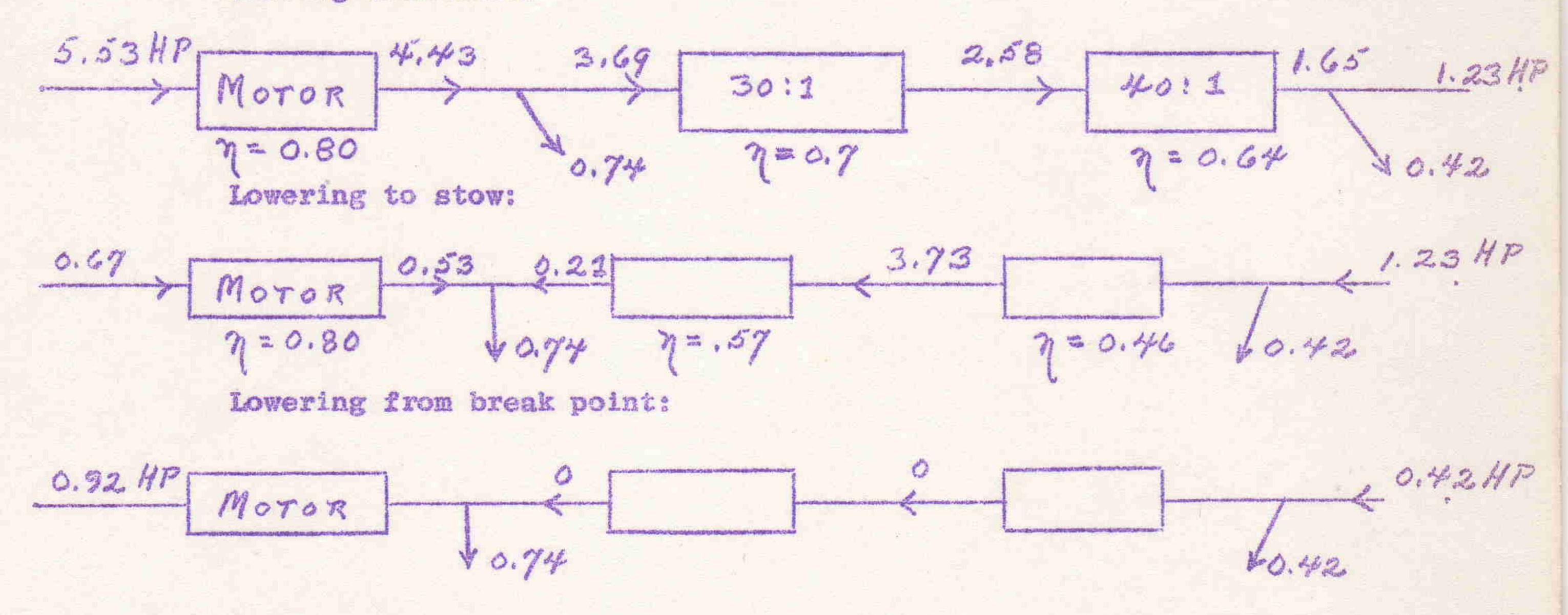
Relief to motor, from breakpoint to stow = 0.92 - 0.67 = 0.25 HP = 0.19 KW Runaway point:
