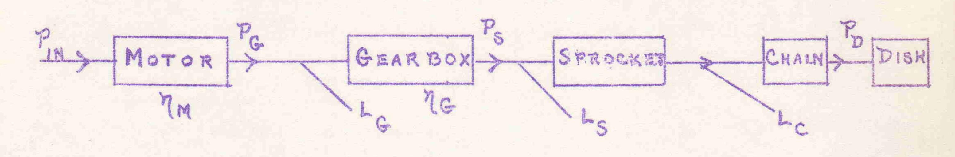
P<sub>IN</sub> = electrical power to motor
