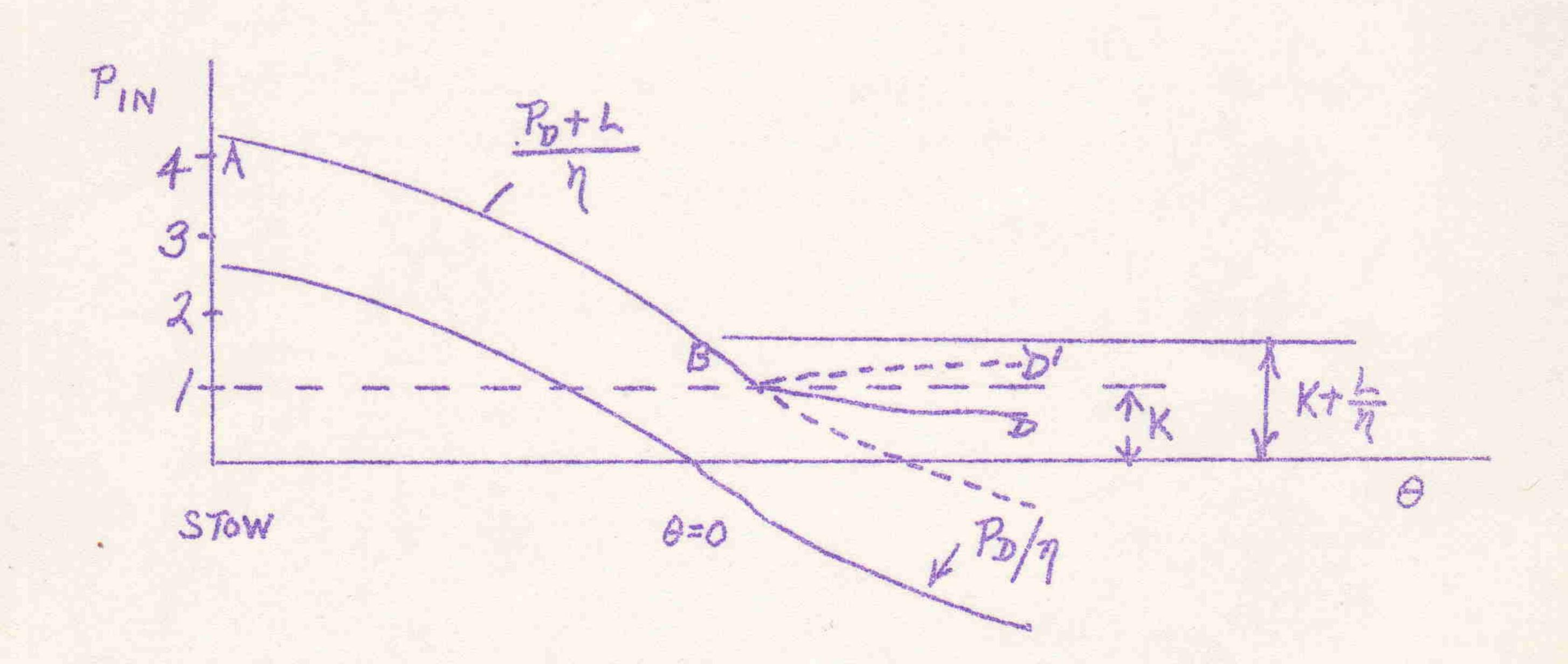
The expected curve is ABCD. At B, where the dish is balanced,  $P_{IN} = K + L/\gamma$ , so power is still required to move the dish. At C, where  $P_D + L = 0$ , only the power K is required. On the segment CD,  $P_D + L$  is negative so that motion of the dish feeds power back into the gearbox. Then Eq. (3) applies. Now  $\gamma_{REV}$  is negative for a self-locking gearbox; the more the dish helps the harder we have to work to lower it (CD'). (See Appendix 5.)
